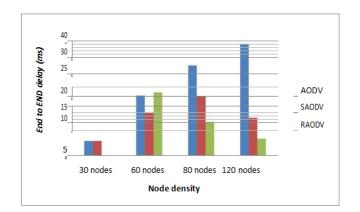
Figure.2: End To End Delay under AODV, RAODV and SAODV
